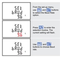
On completion of the entry procedure, press [ to confirm the setting and press [VAT] to return to the main set up menu.
