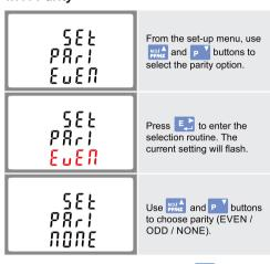
On completion of the entry procedure, press to confirm the setting and press WAT to return to the main set up menu.
